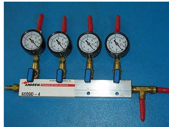
Figure 9.3 System manifold example
